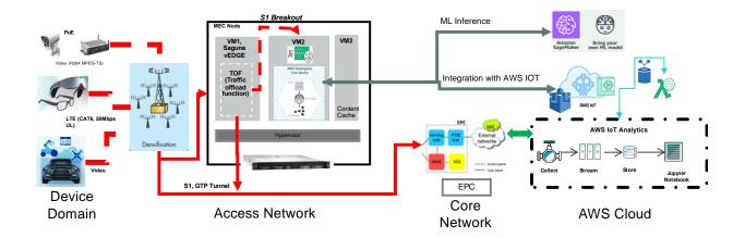
This design approach, based on the Mobile Edge Platform, enables cost efficient way of building and operating Smart City Surveillance system, with edge processing for bandwidth-hungry and latency sensitive services.
