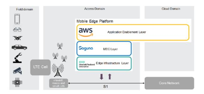
The proposed Mobile Edge Solution consists of three main layers as illustrated above:
